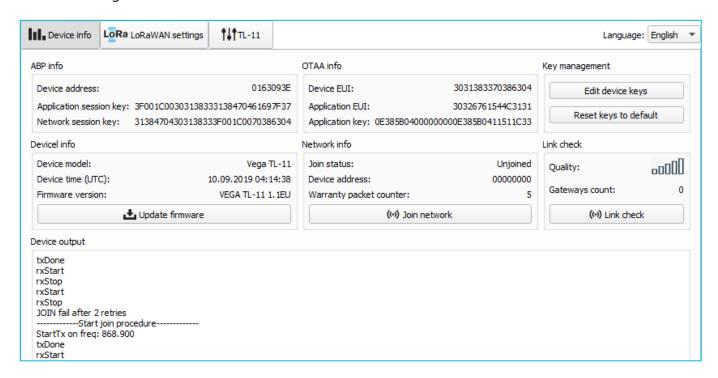
**ABP info** - displays the data necessary to register the device in the LoRaWAN network with ABP method (Activation By Personalization).
