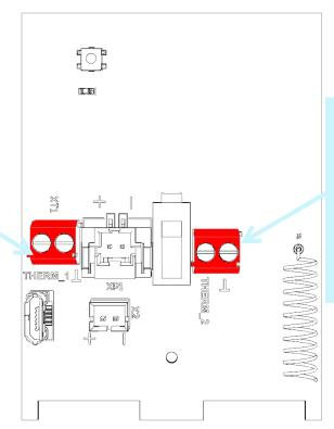
Contacts for connecting external probe
