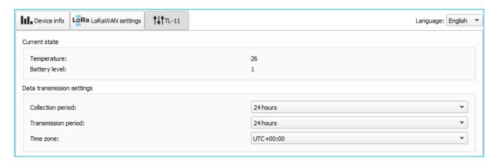
**Current state** – displays the current parameters of the device - the internal temperature of the device and the battery level.
