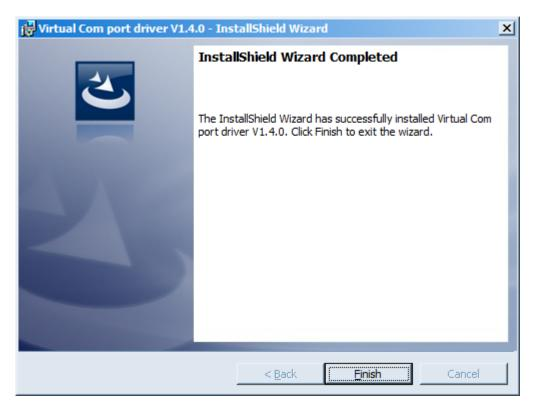
After pressing **Finish** the driver is ready for operation, - it is possible to connect the device via USB.
