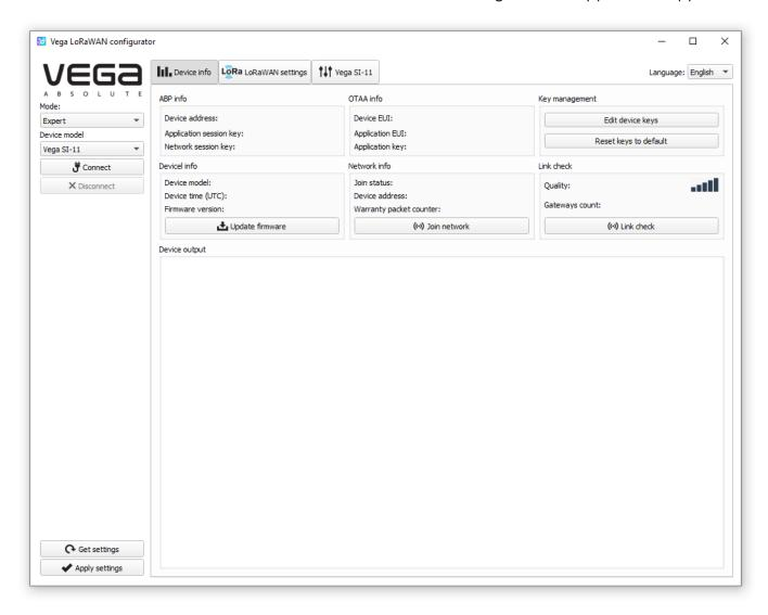
The menu on the left allows you to switch between the "Simple" and "Expert" modes, select the device model, connect to the device or disconnect from it, get and apply settings.
